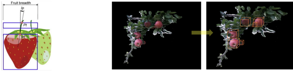
(a) Peduncle angle calculation from the geometry of strawberry [48]. (b) Apple recognition result in point cloud from [126].
