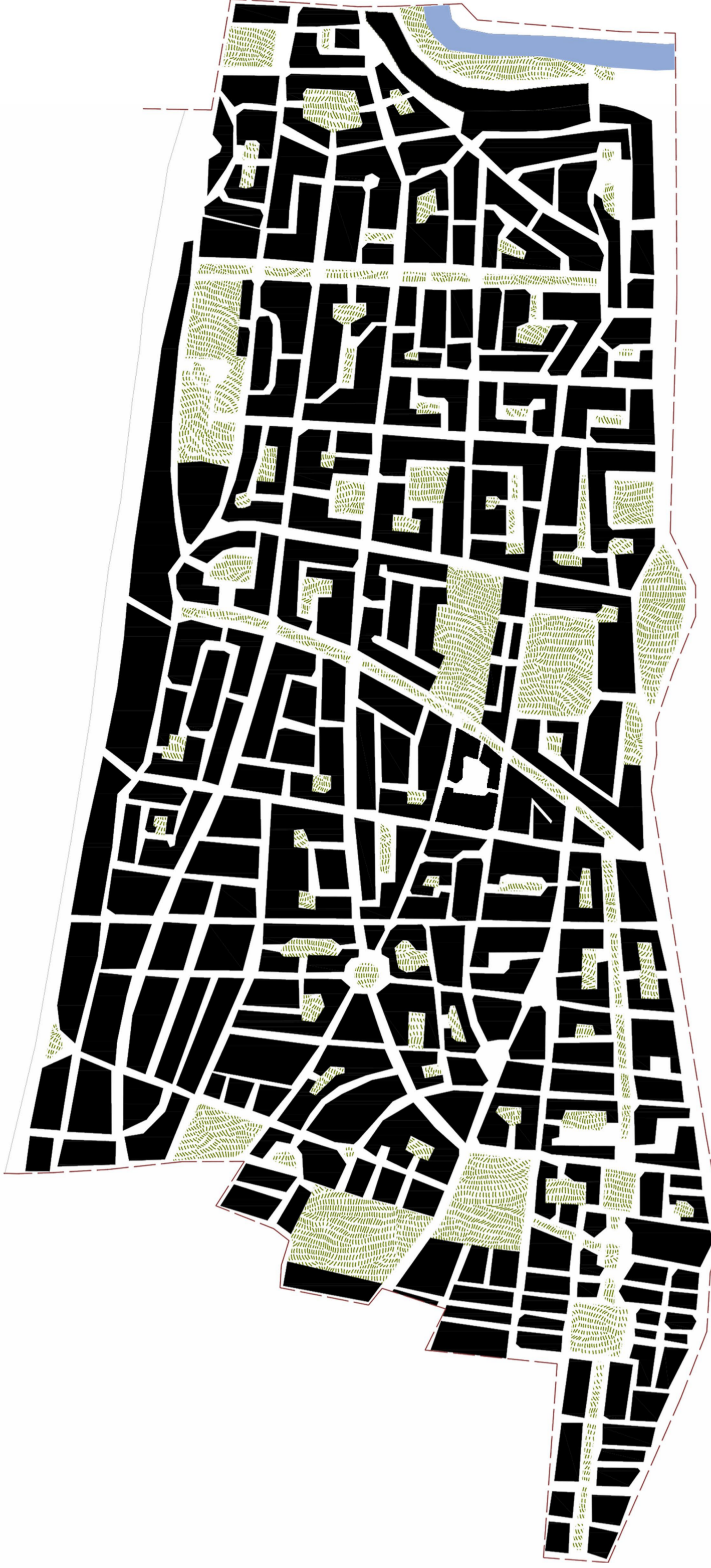
The first Geddes Plan, designed as an adapted version of Ebenezer Howard's garden-city. The urban grid is characterized by the presence of public and private gardens. Geddes planned the roads to favour the flow of sea breeze. The bigger roads are set parallel to the sea (north to south), and the smaller roads from the sea to the inside of the city.
