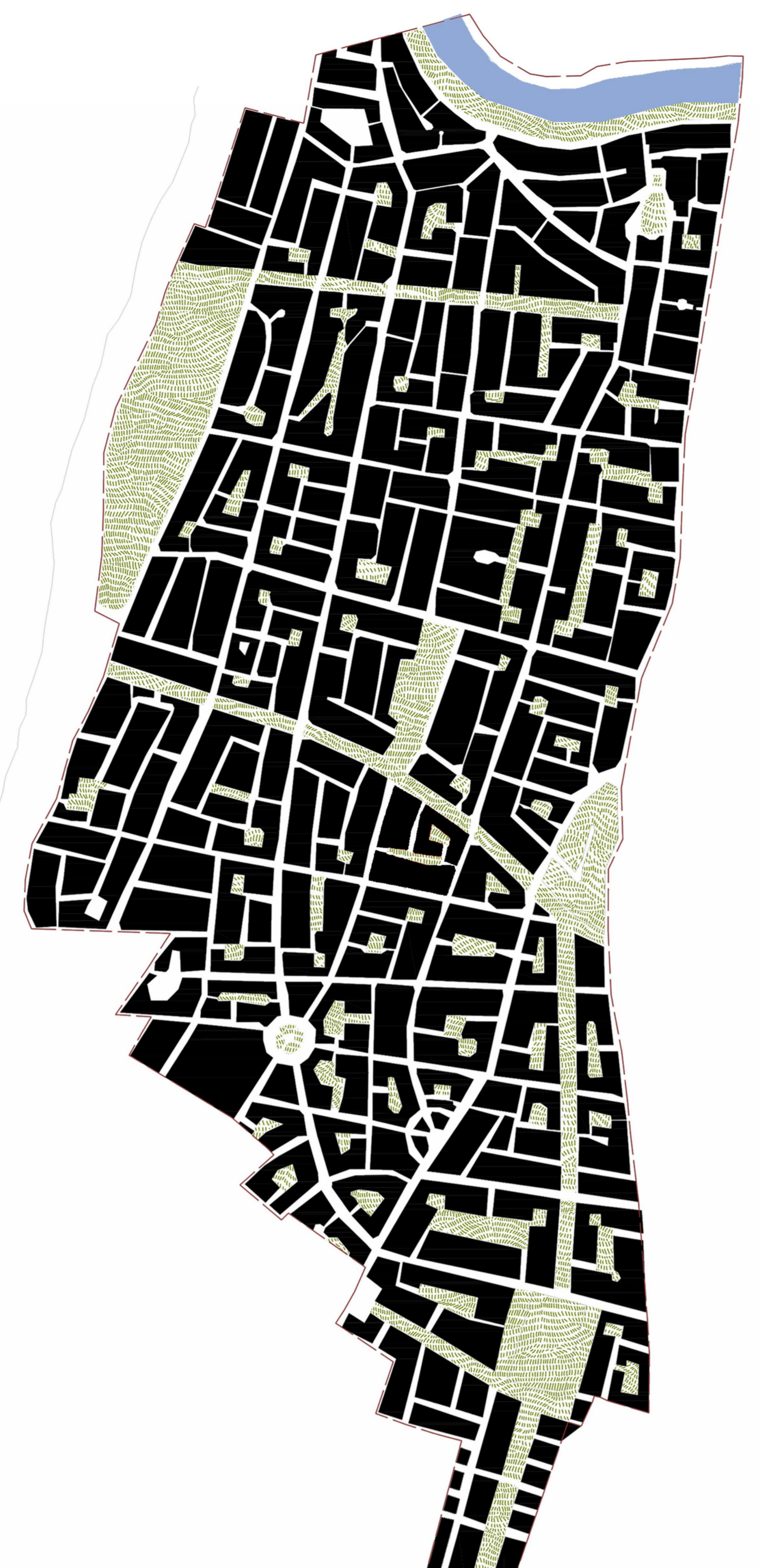
Patrick Geddes' second plan, an edited version of the 1925 plan. The housing capacity increased to 100.000 people due to the growing migration. The green areas were reduced, the same for the distance between buildings.
