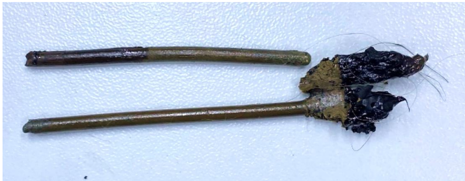
Figure 63. Colour change after degradation
