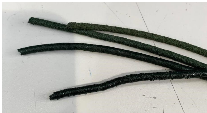
Figure 39. Irregular filaments from initial parameters set
