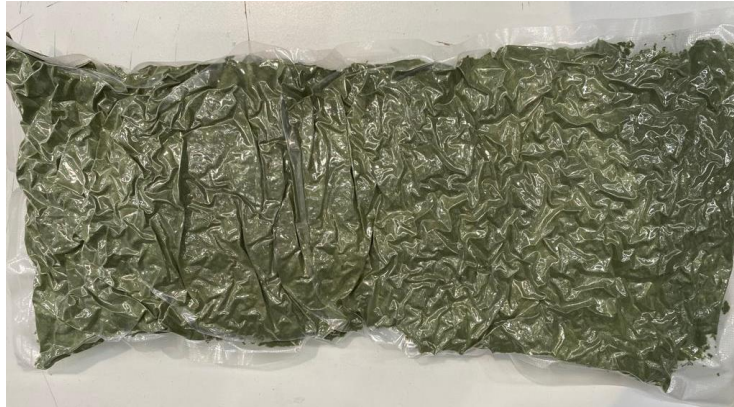
Figure 24. Vacuum sealed grinded and dried nylon fibers
