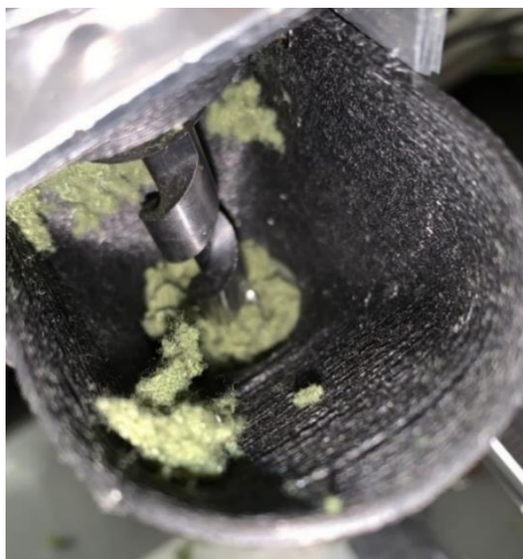
Figure 26. Hopper and screw of the pellet extruder
