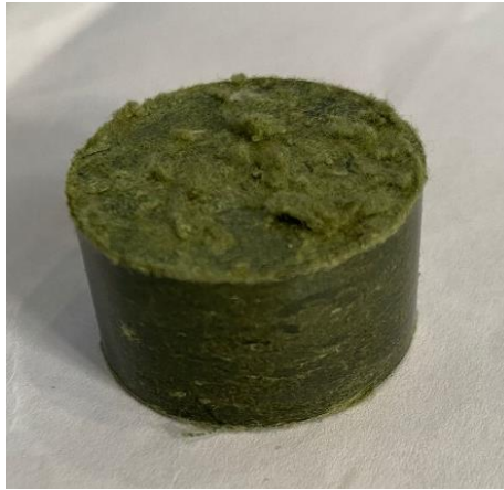
Figure 25. Result of hot mounting process
