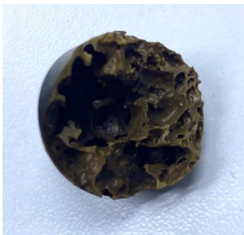
Figure 64. Clogging material inside the nozzle
