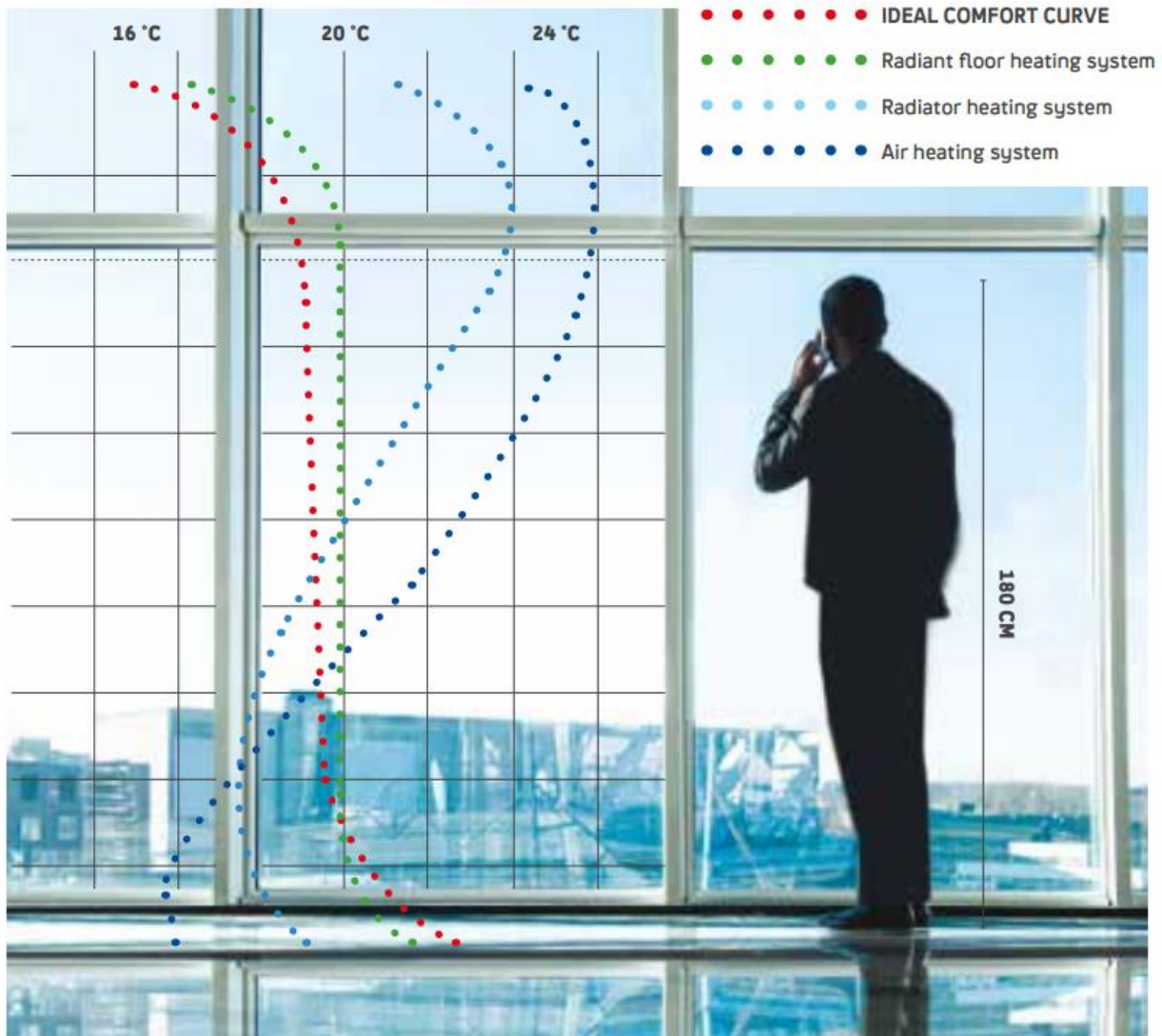
Figure 4- 40 The temperature vertical distribution in a radiant floor system follows a comfort curve very close to the ideal
