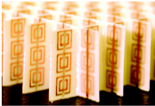
Figure 1.10: Architecture of Smith et al. [37] for the first NIM. The red squares represent the resonators, deposited on fiberglass, and the vertical stripes running through the squares are the wires. Taken from [37].
