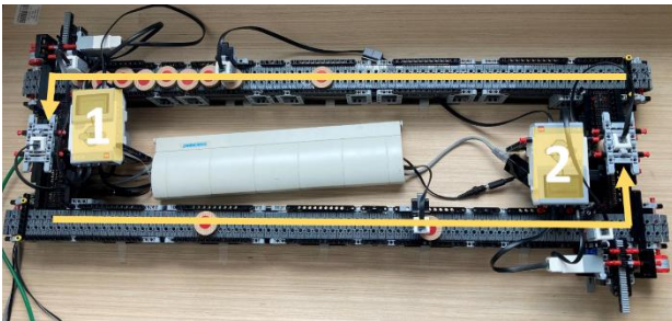
Figure 3.4: Lab-scale model: 2-station closed-loop system
