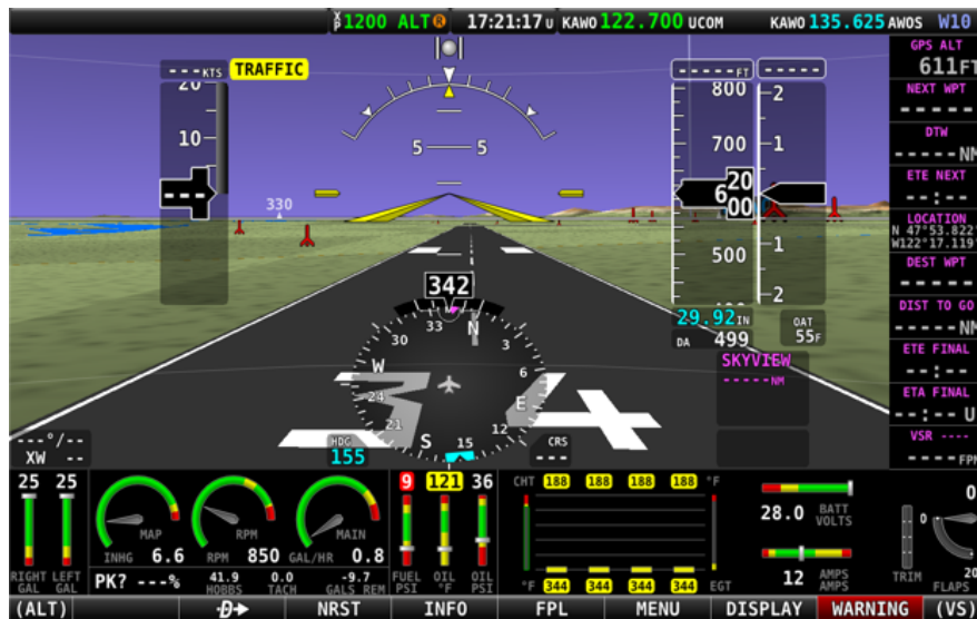
Fig. E.4: Dynon SkyView HDX PFD example view [35]
