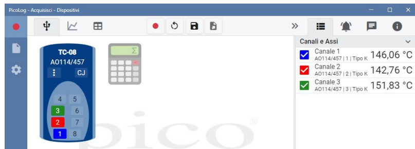
Figure 32: PicoLog 6 main software screen - multiple connected thermocouple
