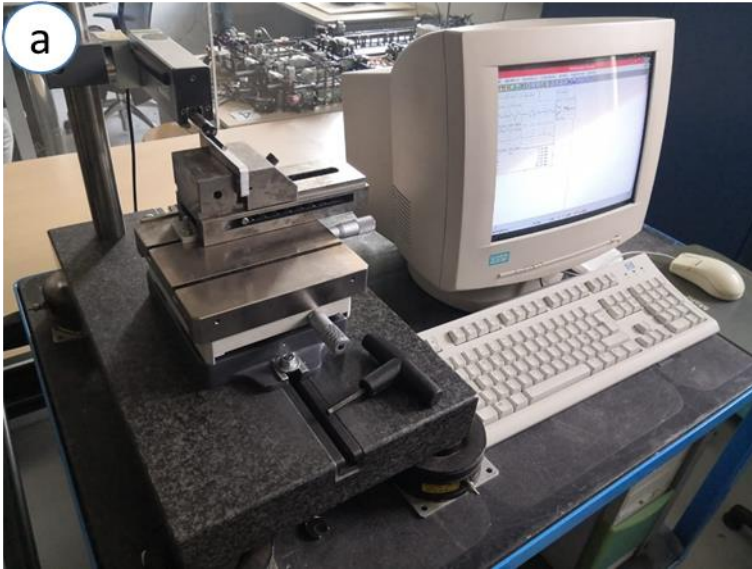
Figure 40: Mahr Perthometer PGK (a) – Contact stylus with 5 \mu\text{m} tip MFW-250 (b)
