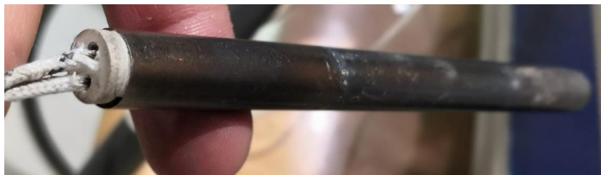
Figure 48: Cartridge electric resistance heater
