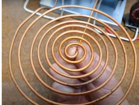
Figure 49: Induction “Pancake” coil example (to be implemented in the laser machine)
