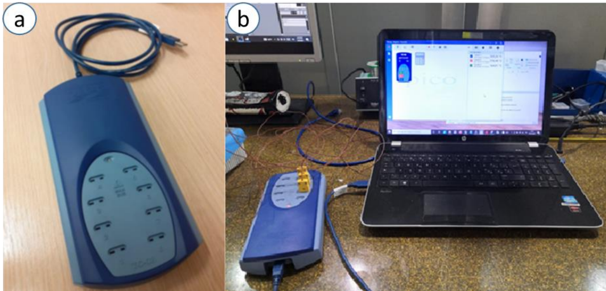
Figure 31: TC-08 datalogger (a) - Thermocouples connected to the datalogger, connected to the elaborator (b)
