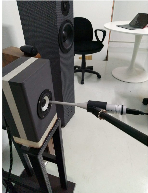
Figure 1: Frequency response near-field measurement of a TMAUDIO R2c system
