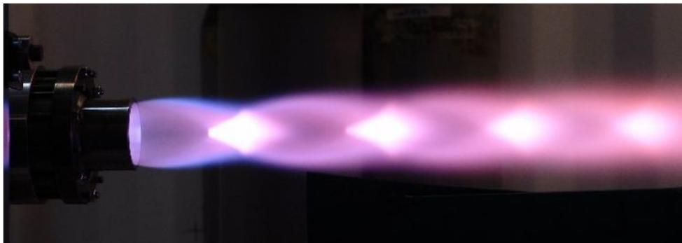
Figure 2.5: Overexpanded jet during a SpaceX Raptor Engine Test.
