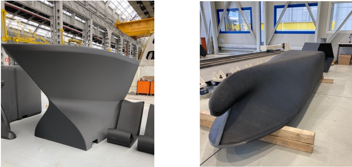
Figure 10a & 10b – Additively manufactured mold for naval sector (left) and prototype for hydrodynamic tests (right) – courtesy of Camozzi Group
