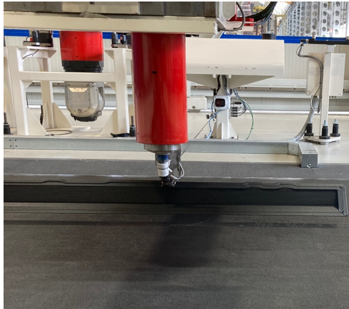
Figure 49 - Printing of the decorative panel, it is noticeable the double-bead structure
