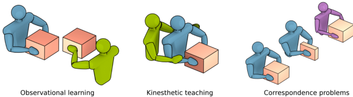
Figure 1.1: From left to right: observational learning, where the cobot uses a vision system to watch the demonstration; kinesthetic teaching, where the cobot is physically moved by the operator; correspondence problem, for cobots with different embodiments and boxes of different sizes
