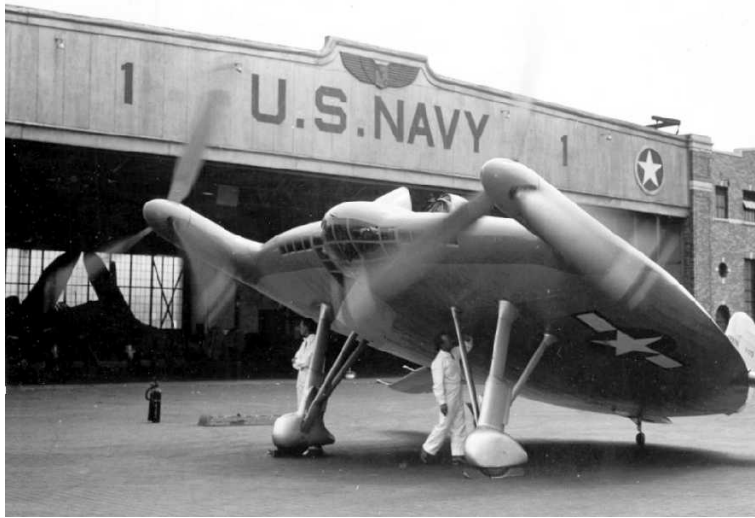
Figure 2.7: Vought V-173 "Flying Pancake", a first application of the WTP.
