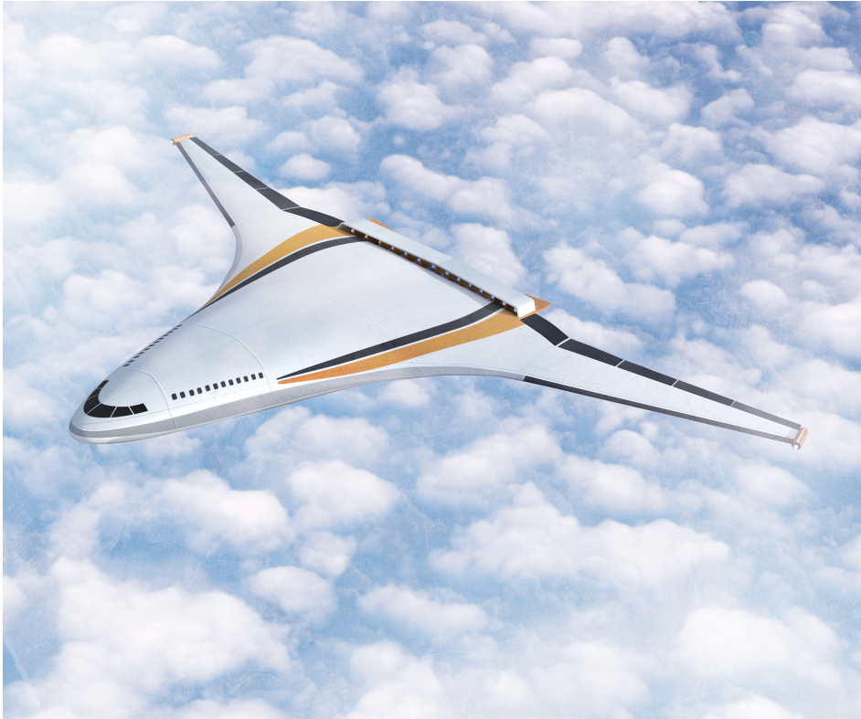
Figure 2.1: NASA N3-X, of interest the adoption of a BWB layout with DEP on the back to exploit also BLI [11].
