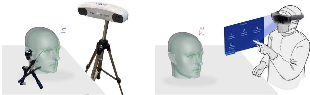
(a) Fiducial points position acquisition using Optical Tracking System. (b) Fiducial points position acquisition using HoloLens 2.
