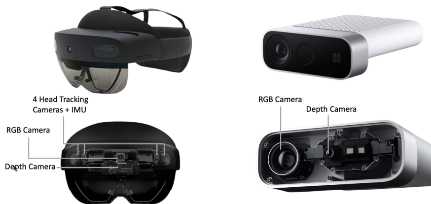
Figure 3: On the left, HoloLens 2 (up) and a breakdown of its main components (down). On the right, Azure Kinect (up) and a breakdown of its main components (down).
