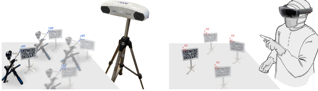
(a) QR Code position acquisition using Optical Tracking System. (b) QR Code position acquisition using HoloLens 2.
