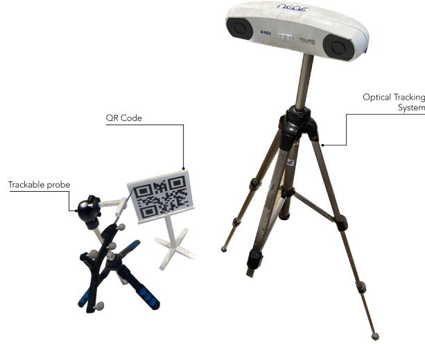
Figure 13: Setup for registration accuracy assessment. An Optical Tracking System (NDI Polaris Vicra) with a trackable probe was used together with a QR code. As long as the probe is in range with the IR field of the system’s receptor its location in the Optical Tracking system reference frame can be retrieved.
