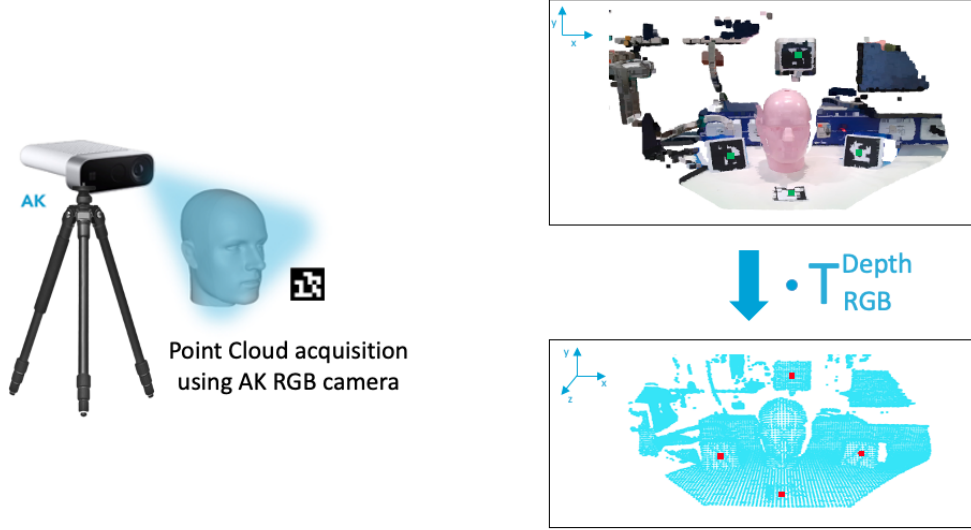
Figure 11: On the left, a practical example of point cloud acquisition using the head phantom and an Aruco marker. On the upper right, a 2D point cloud acquired using the RGB camera of Azure Kinect; green points indicate the detected position of the Aruco markers in 2D. On the lower right, the acquired 2D point cloud is transformed into depth camera's coordinate reference frame by adding the z coordinate, with corresponds to the depth information; Aruco markers in this point cloud are indicated in red.
