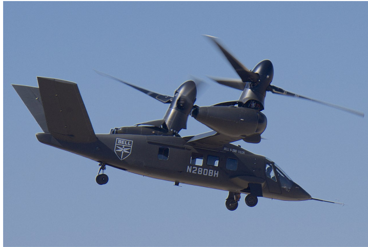
Figure 1.5: Bell V-280, FVL prototype, in hover configuration [4]
