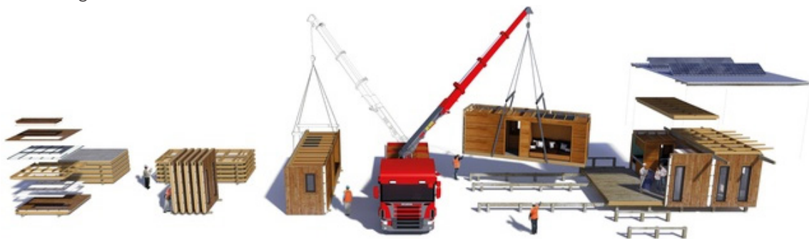
Fig. 33. Graphical Abstract combination of 2D and 3D modular construction. Source: https://www.mdpi.com/2071-1050/8/6/558
