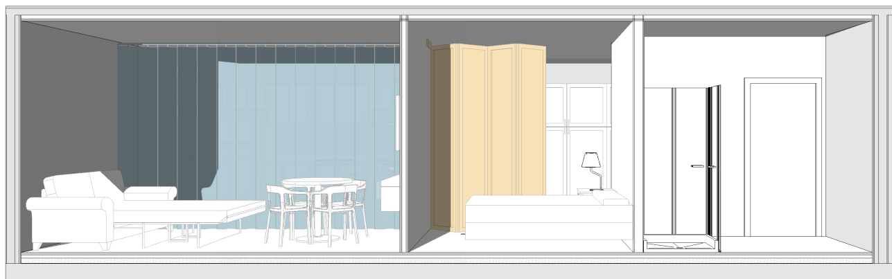
Fig. 102. Module C, interior flexibility proposal, curtain division.
