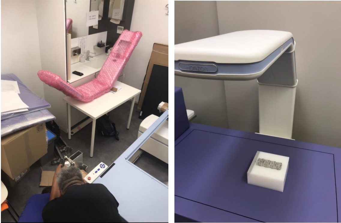
Figure 55: C-arm mounting on DEXA apparatus (a). Phantom Calibration (b).
