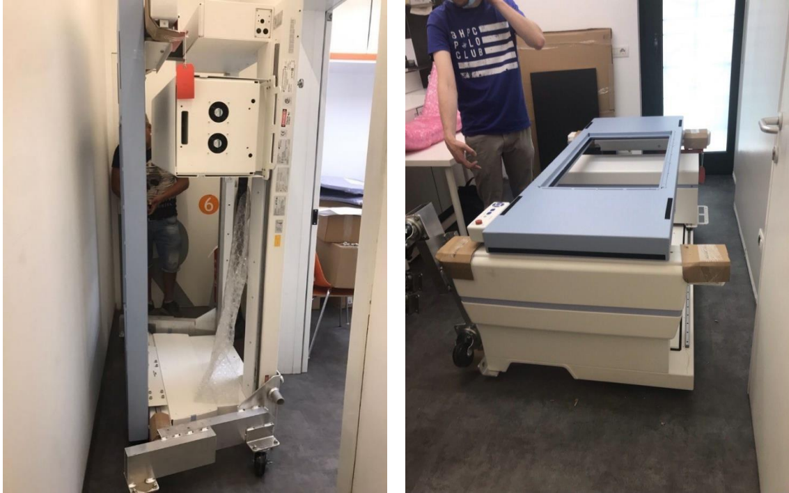
Figure 54: Vertical positioning of the machine with wheels for transportation (a). In room machine positioning (b).
