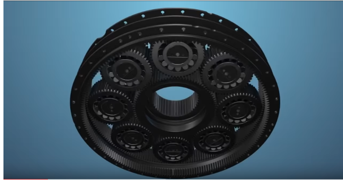
Figure 4.1: Schematic representation of an epicyclic gearbox stage [2]
