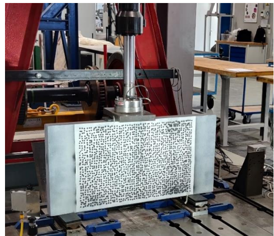
Figure 3.2: xps pre-cracked panel with painted speckle
