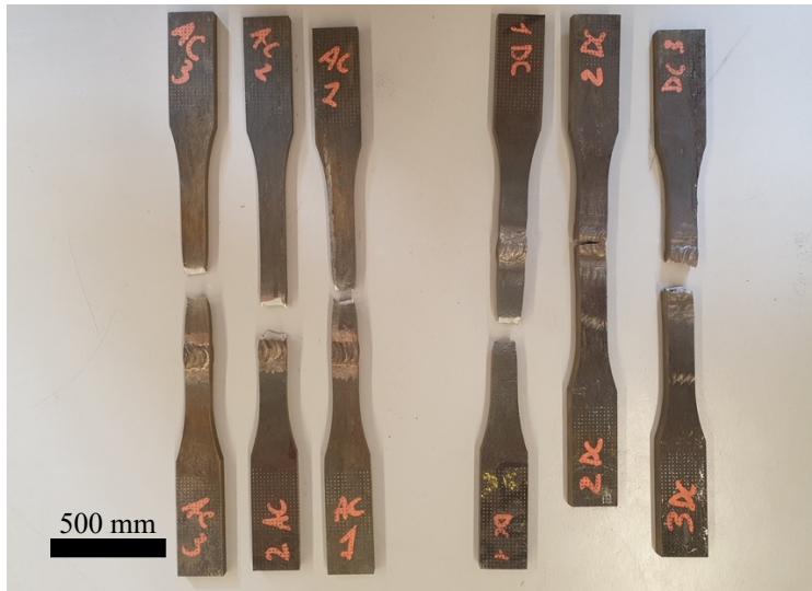
Figure 95: The tensile tests specimens after the failure
