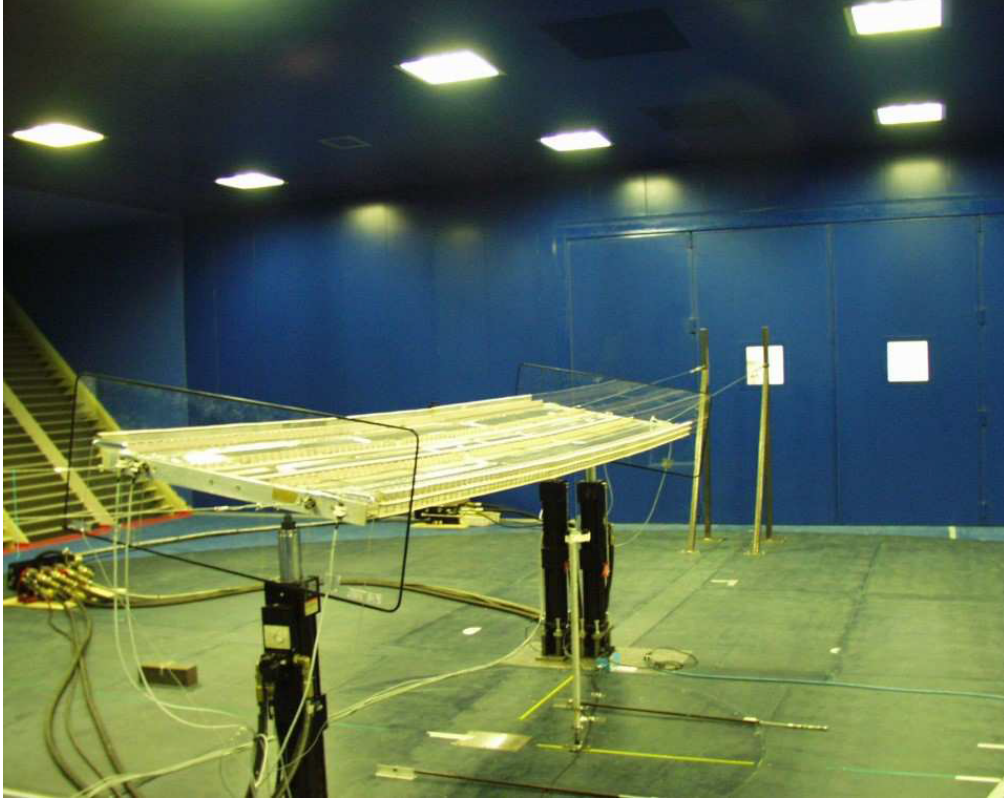
Figure XX: Forced motion testing on a deck sectional model
