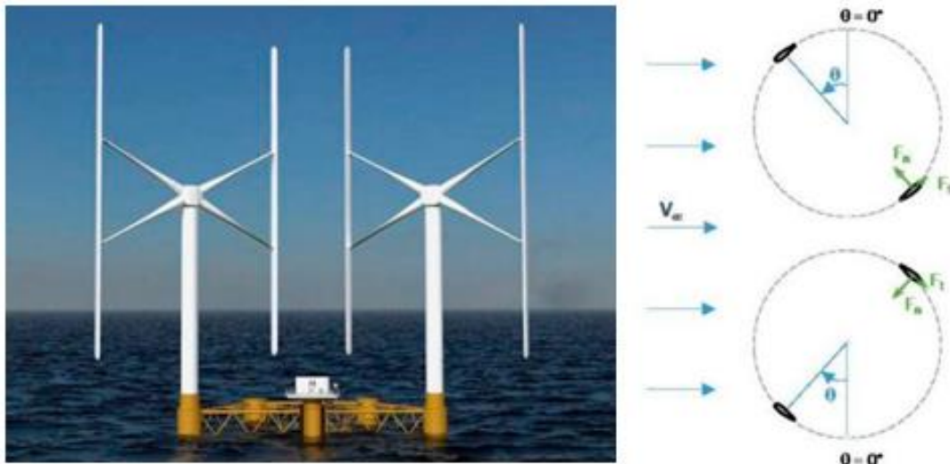
Figure 2.11 – Rendering of the double turbine configuration and its schematics studied in [36].
