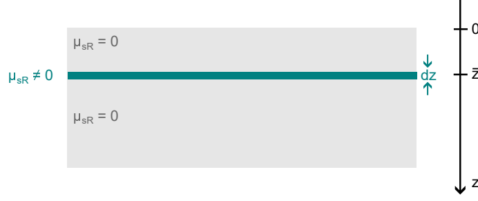
Figure 2.3: Schematic representation of the approach used in our calculation about the generation depth of detected Raman photons
