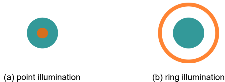
Figure 3.9: (a) point illumination scheme, (b) ring illumination scheme. In orange we have the illumination region while in blue the collection region
