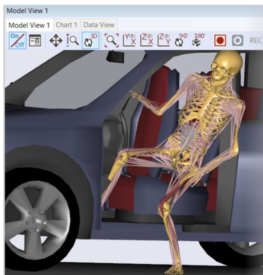
Figure 6 Musculoskeletal model getting out of a car. Source: AnyBody Modeling System. https://www.anybodytech.com/software/ams/
