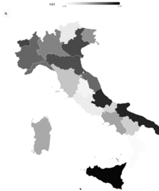
Figure 5.5 – Average time needed to pay-back the additional emission embedded in Medium BEV with respect to same segment ICEV by region.
