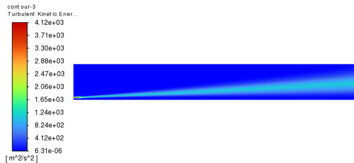
Figure C.9: Color plot: turbulence kinetic energy
