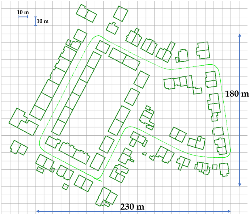
Figure 4.1: Overview of the sequence used map from OpenStreetMap and its trajectory. A square represent a 10 \times 10 \text{ m}^2 area. The trajectory is distributed on a total area of approximately 230 \times 180 \text{ m}^2 , for a total length, estimated by the scan matching, of 687.116 m.
