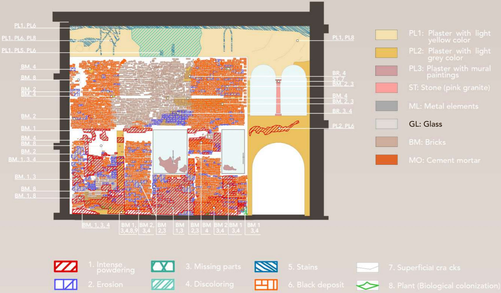
MATERIAL AND DECAY MAPPING made by GR05 1/100
