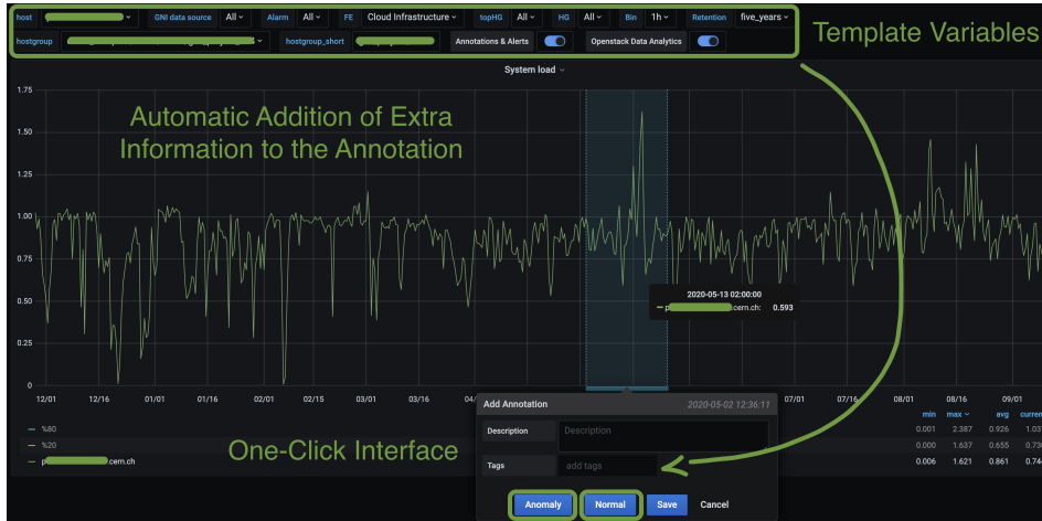
Figure 4.1: Modification introduced in the Grafana Annotation interface. Template Variables are automatically appended as tags.
