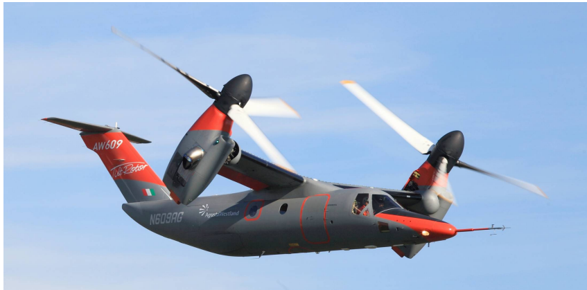
Figure 1.7: AW609 during flight test. Note the tilting system that was designed for rotating all the engine bay
