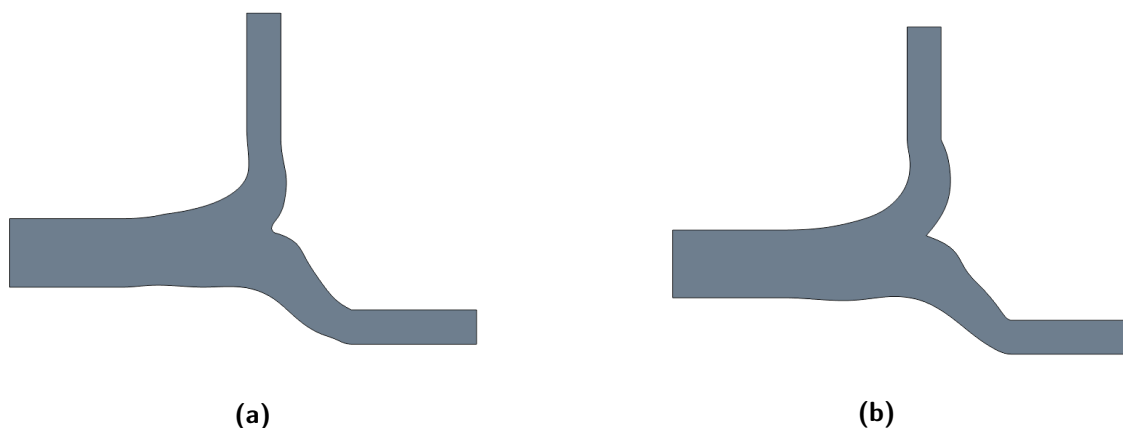
Figure 4.22: Optimized geometry reconstruction - Trim (a) VS Poly (b) mesh models
