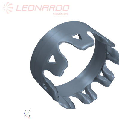
Figure 5.37: CAD model of the optimal solution - Pressure minimization case.
