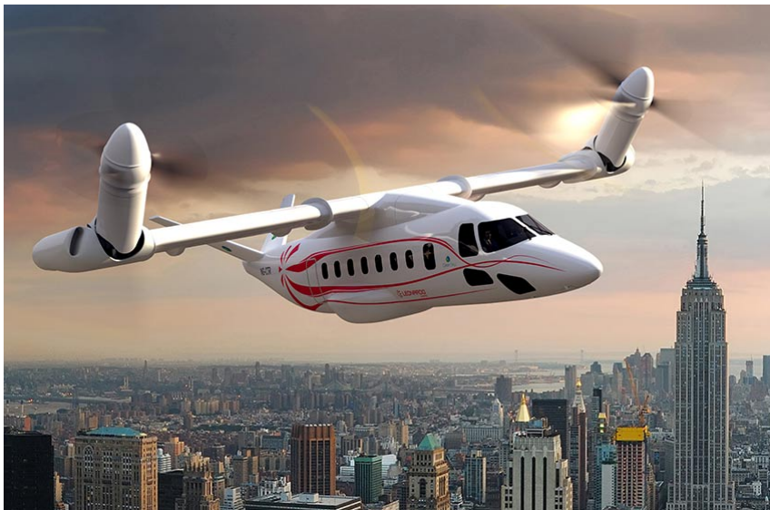
Figure 1.6: Next-Generation Civil TiltRotor rendering. Note the new idea of tilting system with respect to the one of the AW609
