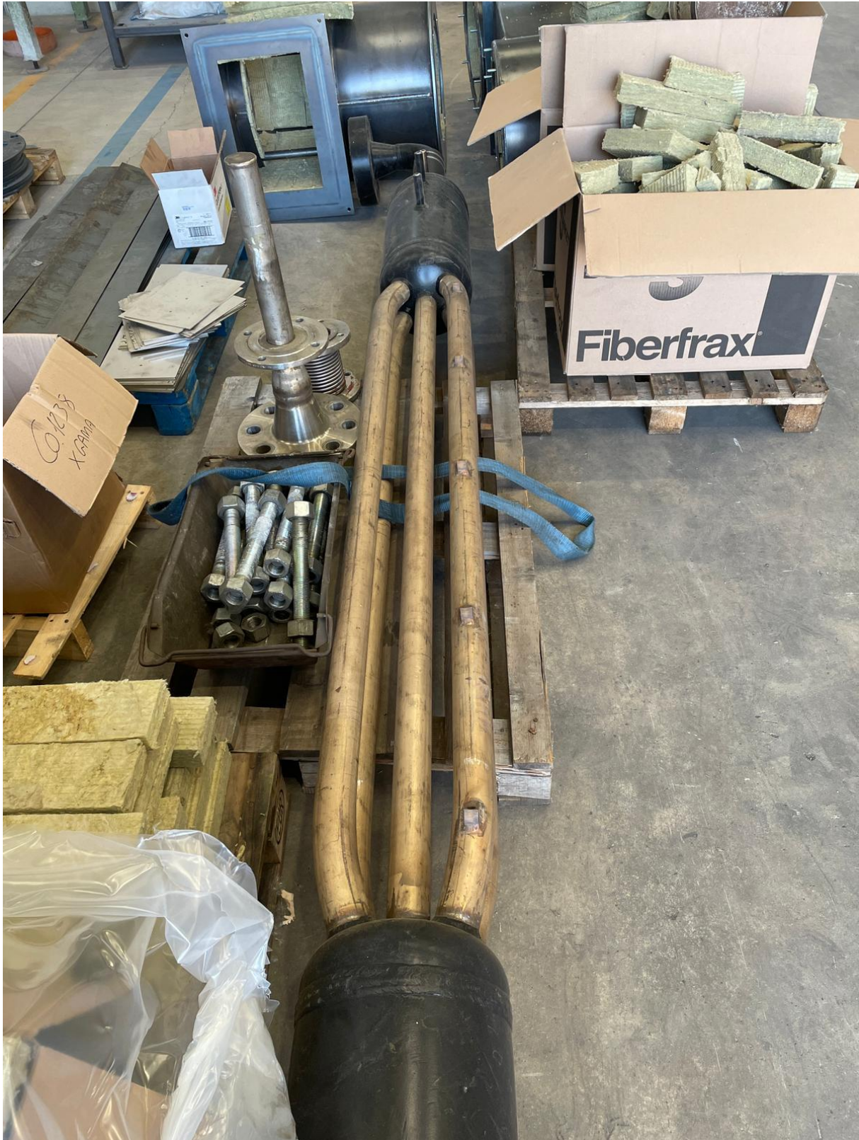
Figure 12: Tube heat exchanger before installation inside the pool
