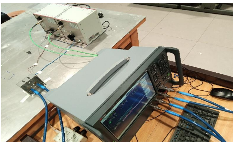
Figure 5.10: Experimental test bench to characterize the LISN.
