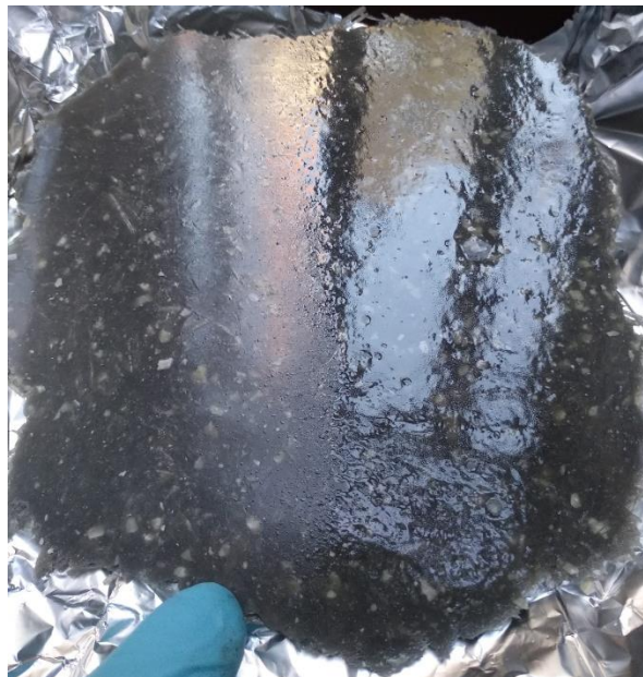
Figure 96. Airbrush coating composite with the solution of AralditeBY158, Phthalic Anhydride and Omnicat440 (3%) with previous pre-treatment surface.
