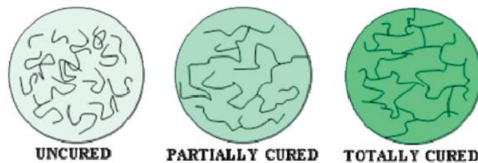
Figure 31. Crosslinking of thermoset molecules during curing.
