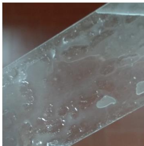
Figure 93. Result of coating with a solution of AralditeBY158, Succinic Anhydride and Omniscat440 (3%).
