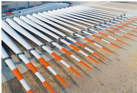
Figure 40. Turbine blades composed by glass reinforced polymer composite.
