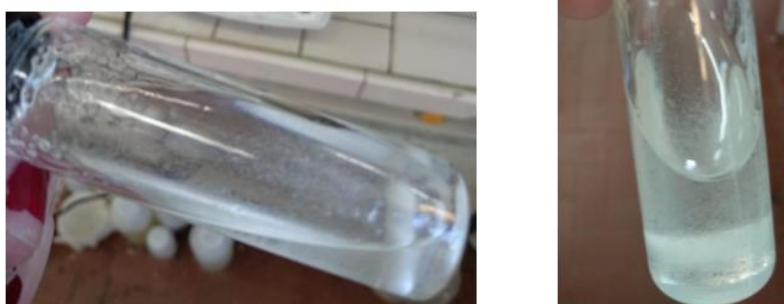
Figure 77. Result of mixing solution of AralditeBY158, Succinic Anhydride and Omnicat440 (3%).
