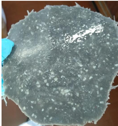
Figure 94. Airbrush coating composite with the solution of AralditeBY158, Anhydride Phthalic and Omnicat440 (3%).
