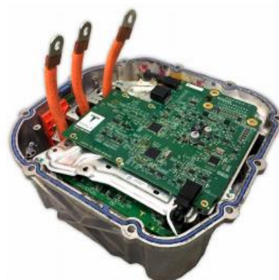
Figure 1.4 Tesla Model S rear drive unit inverter
