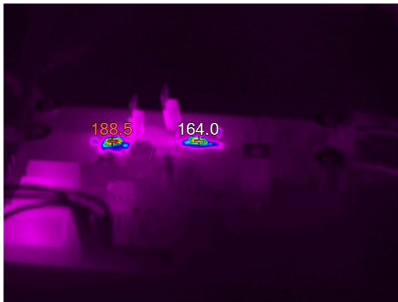
Figure 6.20 Previous snubber circuit temperature Q1 on the left and Q2 on the right
