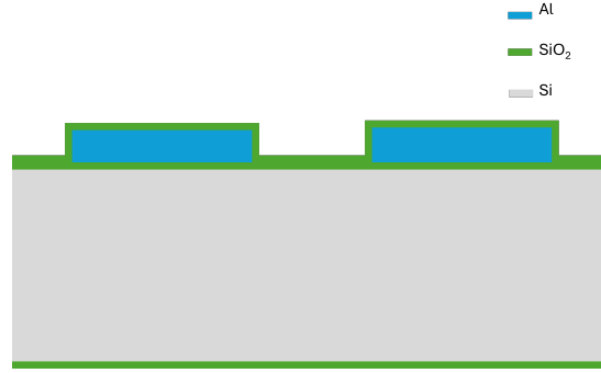
Figure 2.34: \text{SiO}_2 layer uniformly cover \text{Al} shanks of the device.
