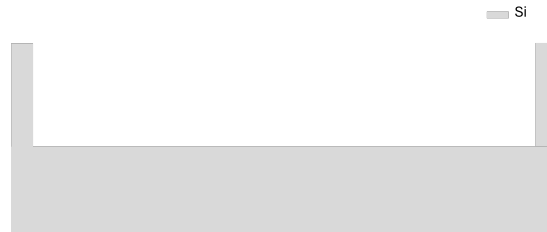
Figure 2.62: Wafer carrier cross section after deep Si etch and PR strip.
