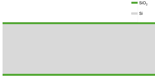
Figure 2.13: \text{Si} wafer section, \text{SiO}_2 present on both sides
