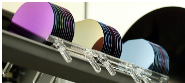
Figure 2.11: 100mm Si wafers, with various layers deposited on top, CMi homepage [68]
