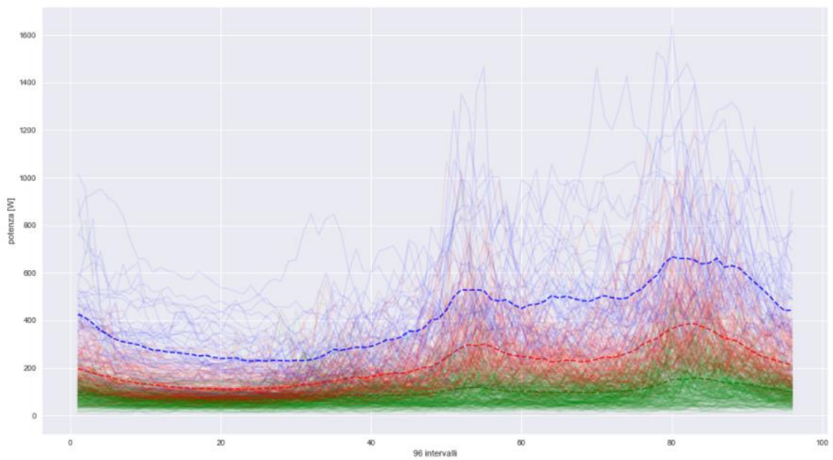
Figure 6-15 – Mean curves of the three clusters and mean power curves of daily (weekdays) power curves of all customers, August.
