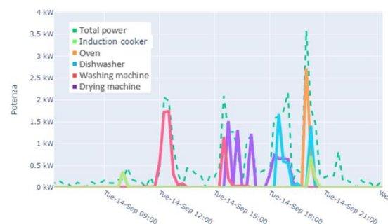
Figure 3-7: Single day power demand of one apartment with details of appliances (14 th of September 2021)
