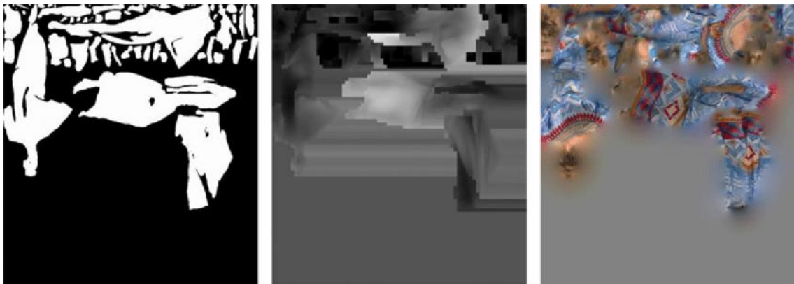
Figure 2.6 - An example of occupancy map (left), geometry (middle) and texture (right) image.
