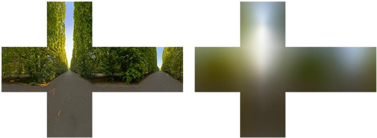
Figure 2.25 - An environment cubemap (left) with the resulting irradiance cubemap obtained by convolution (right)
