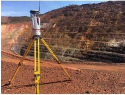
Ground LiDAR mounted on a tripod
