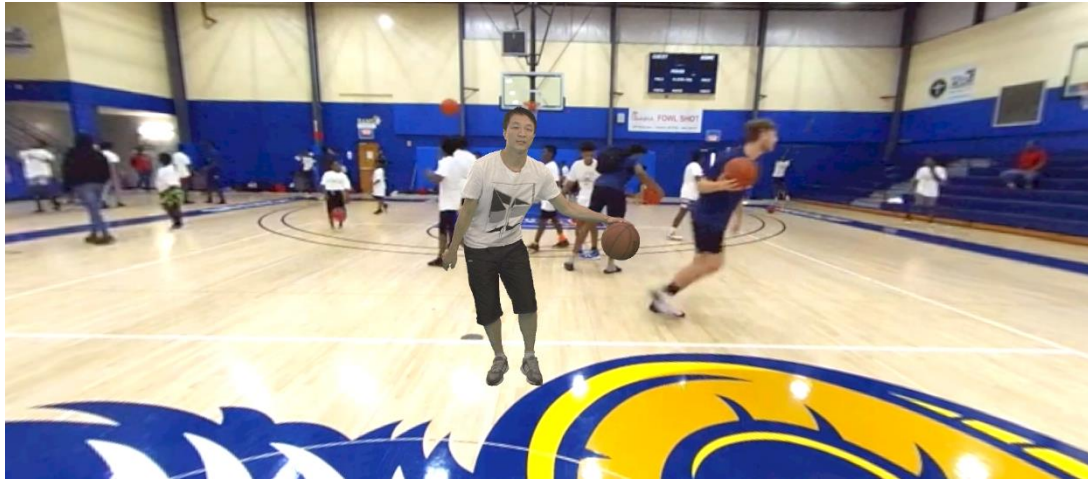
Figure 3.18 – PBR Point cloud model placed in a scene with the indoor 360 video rendered on the skybox
