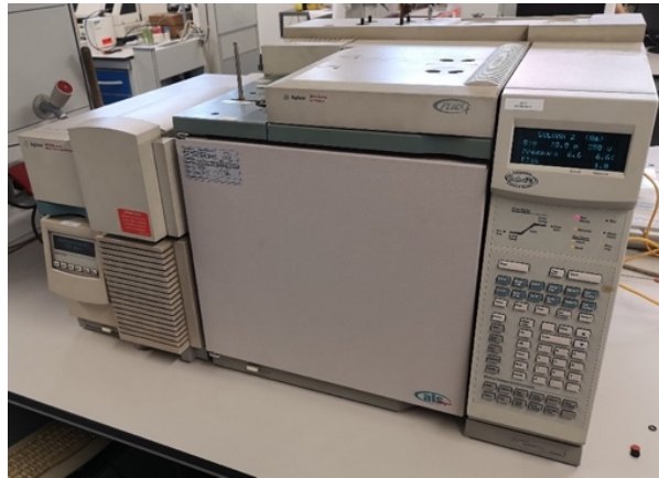
Figure 2.12: Agilent 6890, 5973 MSD Gas Chromatography-Mass Spectrometry with Flame Ionization Detection
