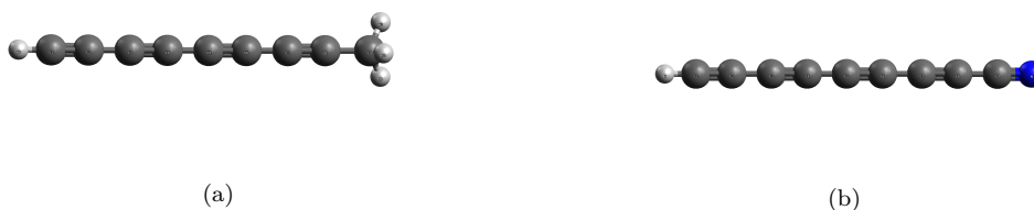
Figure 4.1. Optimized configurations for a)methyl-polyynes, and b) cyano-polyynes. In blue the nitrogen atom.
