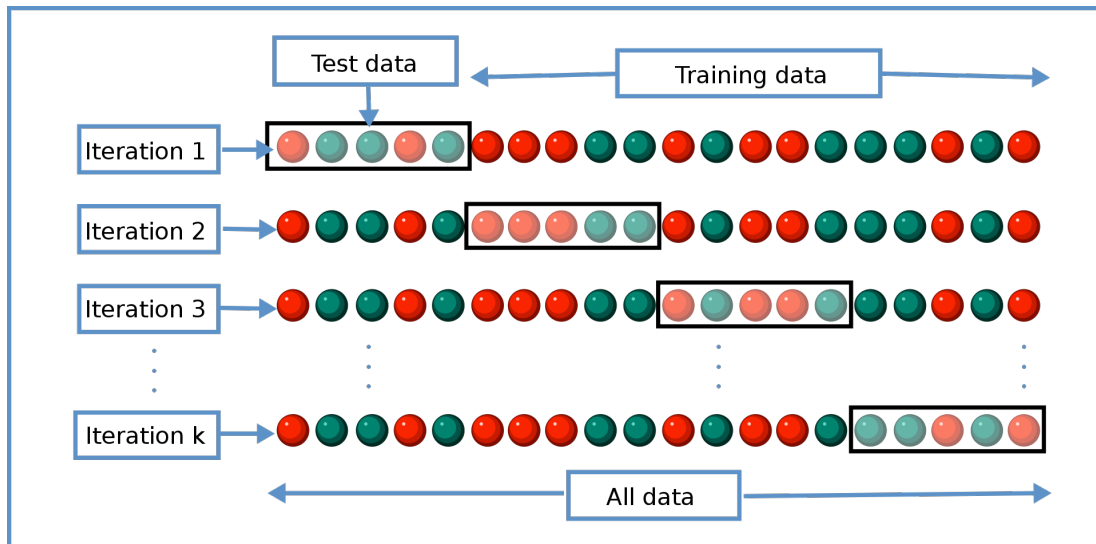
Figure 3.9: Schematization of the cross-validation technique: the entire dataset is divided in a different train and test set for each iteration.
