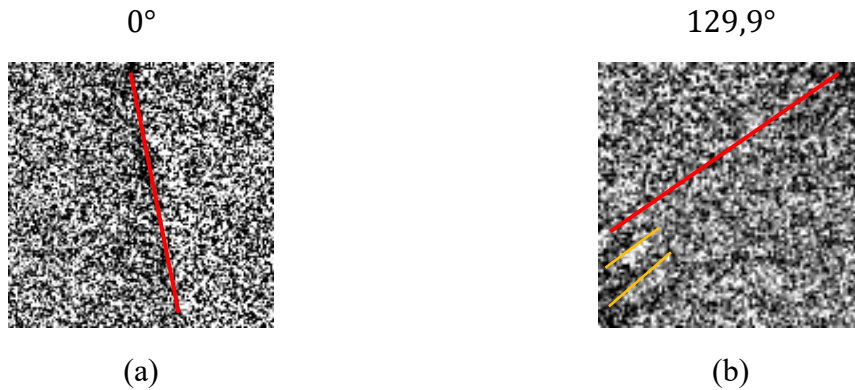
Figure 5.24: example of two frames of time-resolved SoXL measurements at (a) 0^\circ and (b) 129,9^\circ with size 7,5 \mu\text{m} \times 7,5 \mu\text{m} . The border of the stripline is shown with the red line, while the emitted spin waves on the bottom left with the orange lines.
