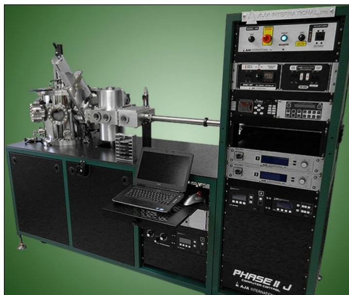
Figure 3.2: The AJA Orion 8 Sputtering System.
