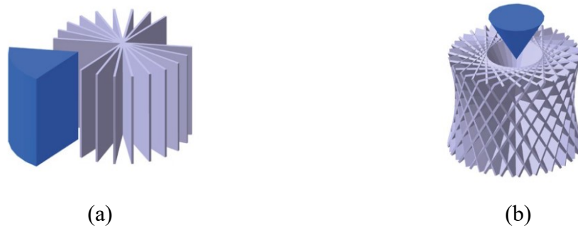
Figure 3.15: (a) Schematic representation of the filling of the Fourier space with the computed tomography setup ( \theta = 90^\circ ) with the corresponding “missing-wedge” artifact: (b) schematic representation of the filling of the Fourier space with the Laminography setup ( \theta < 90^\circ ) with the corresponding “missing-cone” artifact [63].
