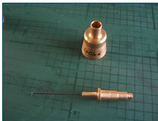
Figure 9.5 — Brass holder and base for the capillary for a high-resolution P-XRD experiment at I11. ( https://www.diamond.ac.uk/Instruments/Crystallography/I11/status/capillaries.html )
