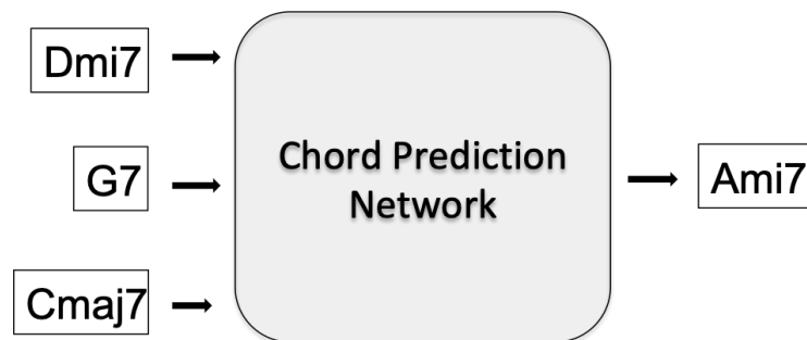
Figure 4.1: Simple outline of the chord prediction problem. Being the transformer an auto-regressive model, it produces one token at a time given all the previous ones and then add the generated symbol to the input in order to further generate new tokens.
