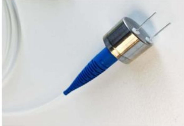
Figure 7 Single transducer cell. Voltage can be applied at the differential leads (pins). Size of the sensing area = 0.3 \text{ cm}^2 .
