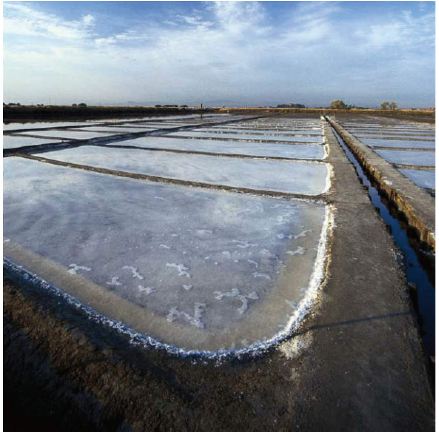
Evaporation ponds in the saltwork of Cervia Source- Parco Delta del Po Archive
