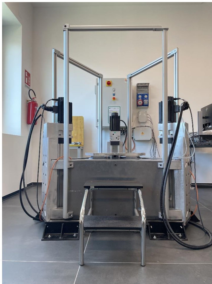
Figure 2.1 Electro-mechanical excitation system
