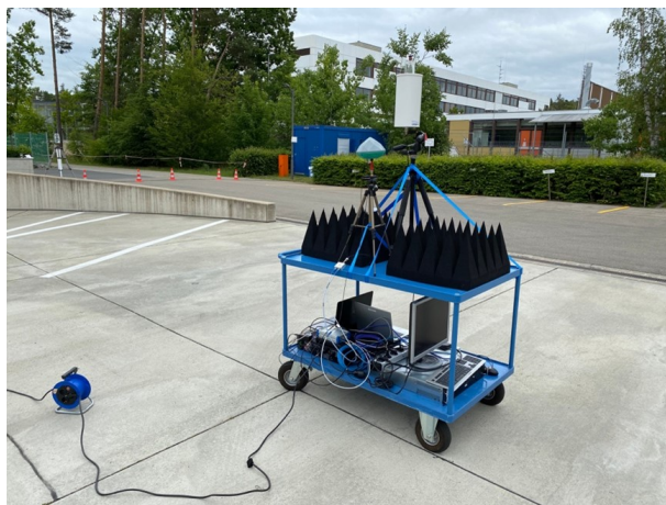
Figure 3.10: Trolley equipped with USRP, Sepentirino and Flexiband receiver for GNSS and 5G NR downlink measurements.[12]
