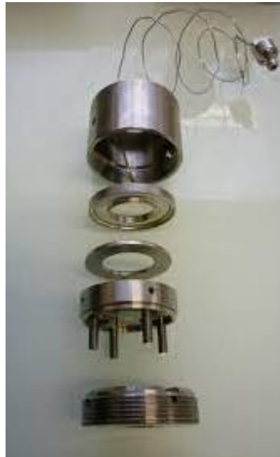
Figure 2.1.1.3: Photograph of a membrane diamond anvil cell.
