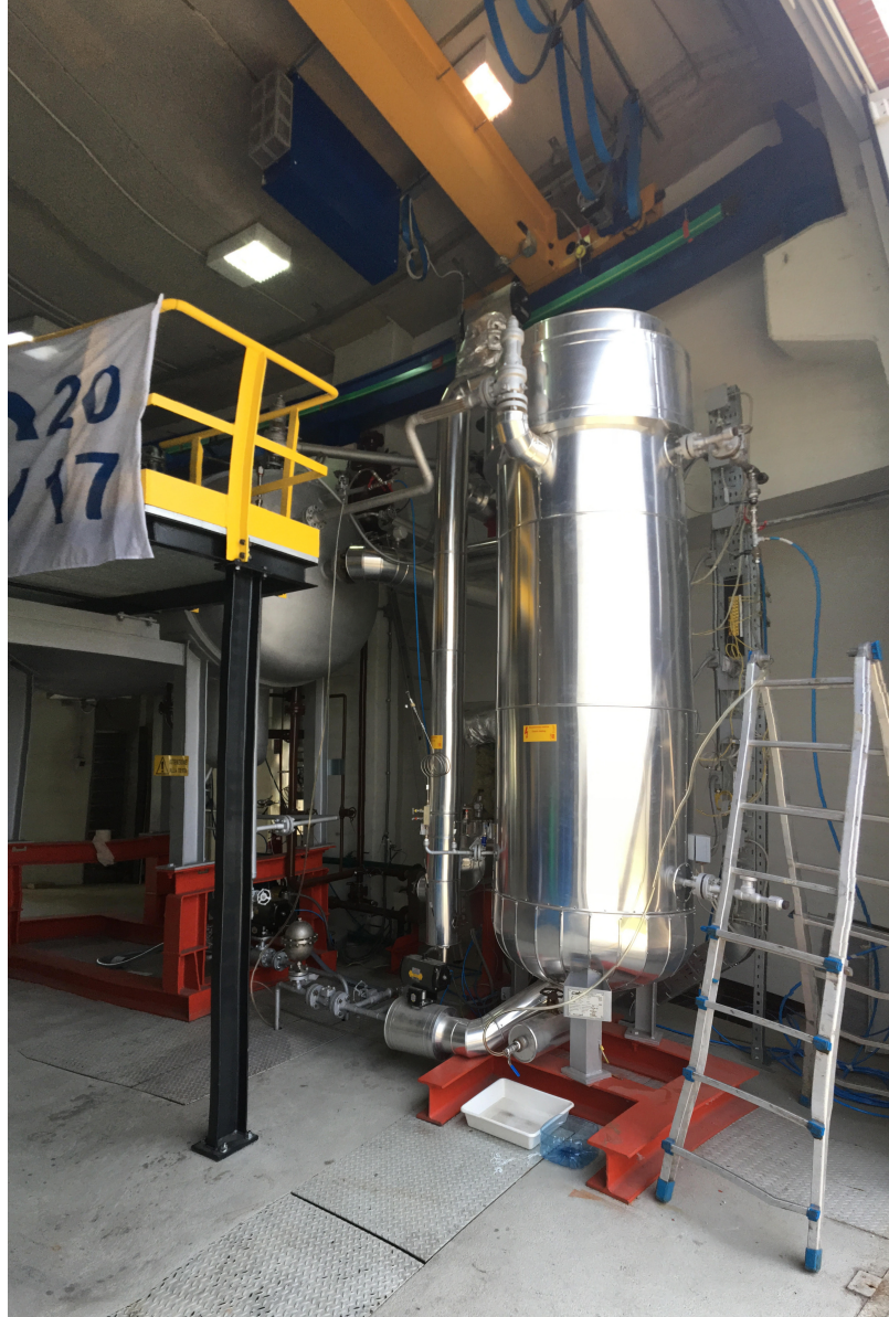
Figure 5.5: The high pressure vessel (on the right) and low pressure vessel (left) of the TROVA.
