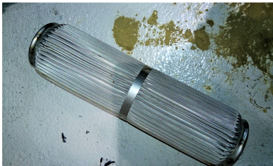
Figure 1.2: Cartridge of the main circuit filter of the TROVA, with the solid residue.
