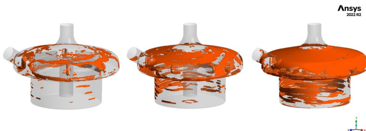
Figura 51: Zone con SS > 50 Pa: (A) NB_PL1 (2500 rpm, 0,5 l/min), (B) NB_PL2 (3000 rpm, 2 l/min), (C) NB_PL3 (3500 rpm, 1 l/min).
